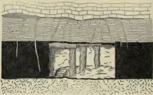
FIG. 14.—Showing Face of Chamber and Gas Working in Roof and Coal
